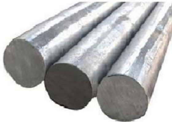
Fig.2. AISI 1040 Steel rods
